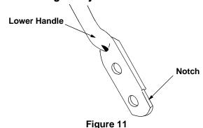
Your mower is shipped with the handle in the higher height position. To lower the handle height, proceed as follows.
